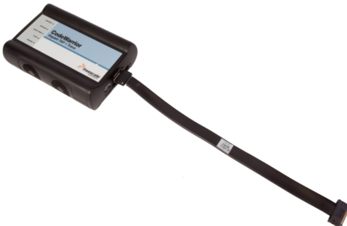
Figure 3-4. Gigabit TAP + Trace probe with aurora nexus cable
