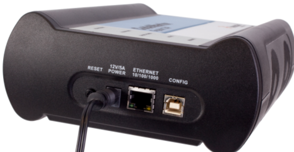
Figure 1-4. Gigabit TAP probe with power cable attached
