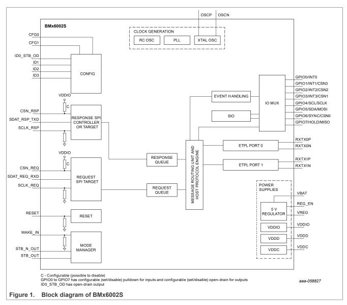
Figure 1 and Figure 2 show the general architecture of the BMx6002 versions.
