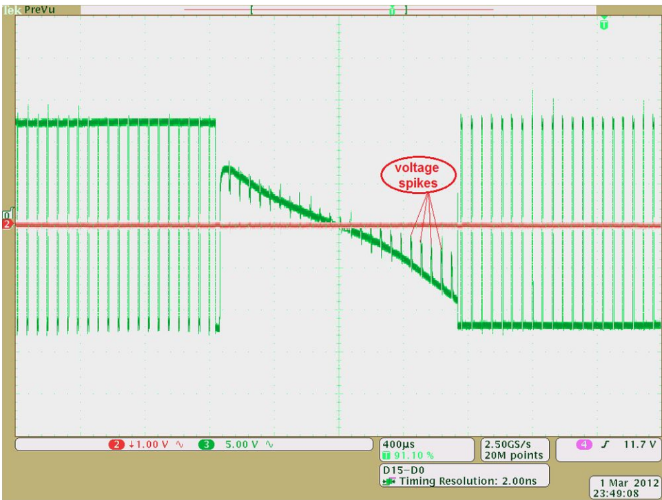
Figure 4-2. BEMF voltage spikes and ADC triggering - A
