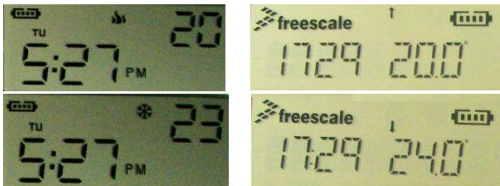
Figure 4-4. Heating and cooling set points
