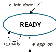
Figure 17. READY state with transitions
